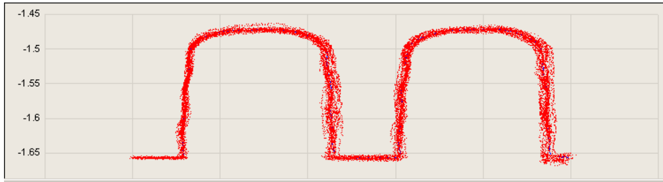
Veeco Dimension X3D resist profile data
